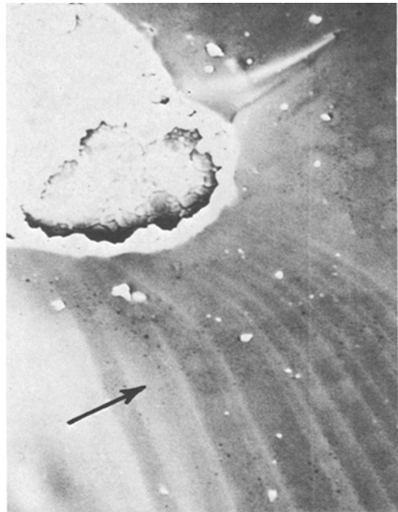
Figure 10 Ni/NiO interfacial failure gives "pseudoporosity" and crack interacts with particle (crack direction arrowed).
