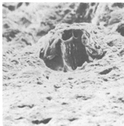
Figure 7 Tilted image of failure of ductile (Al) particle in a glassy matrix (X 200).
